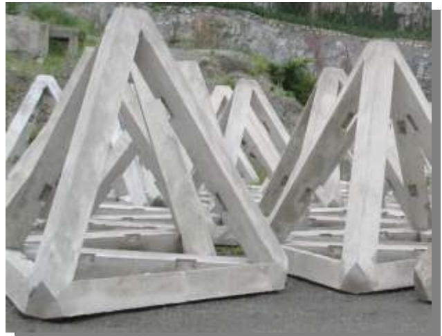
What we may expect to see in Korea. Tetrahedral concrete fish and shellfish modules awaiting deployment.
